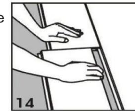
The Released plank can then be pulled out.
